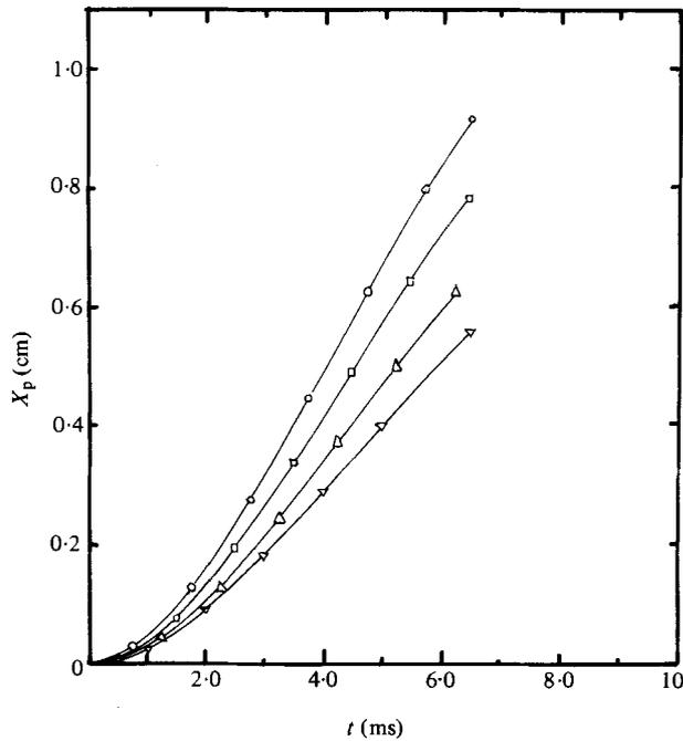
FIGURE 8. Horizontal displacement of different-sized droplets responding to equal-strength N-waves.  $\circ$ ,  $D = 120 \mu\text{m}$ ;  $\square$ ,  $135 \mu\text{m}$ ;  $\triangle$ ,  $167 \mu\text{m}$ ;  $\nabla$ ,  $183 \mu\text{m}$ .
