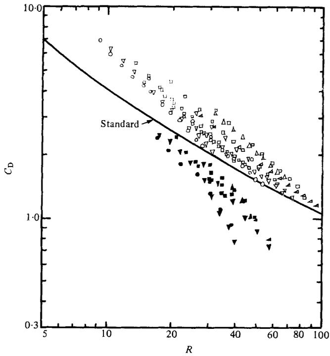
FIGURE 11. Drag-coefficient data. Open symbols,  $dU_r/dt > 0$ ; filled symbols,  $dU_r/dt < 0$ .
