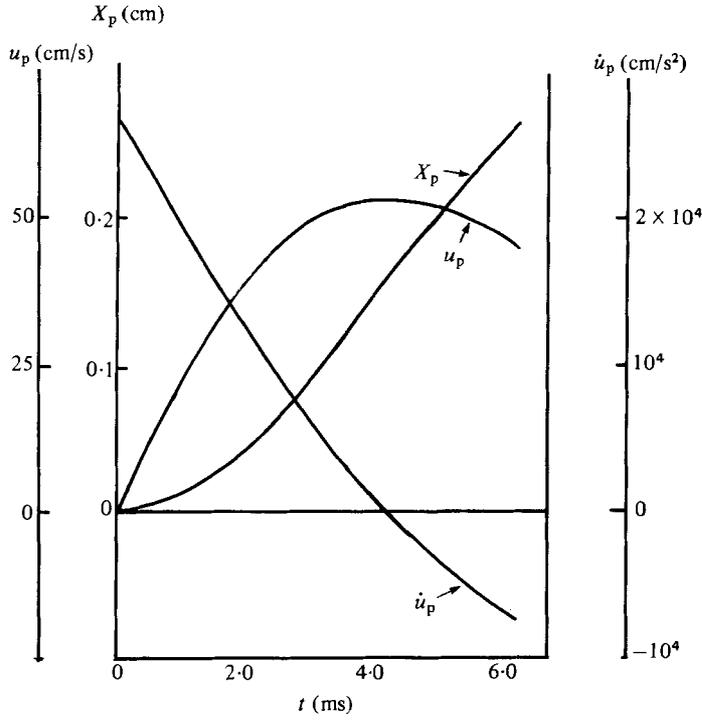
FIGURE 9. Typical variations of horizontal droplet displacement, velocity and acceleration in one test (numerical data for the test shown in the figure, no. 2514, are given in table 2).
