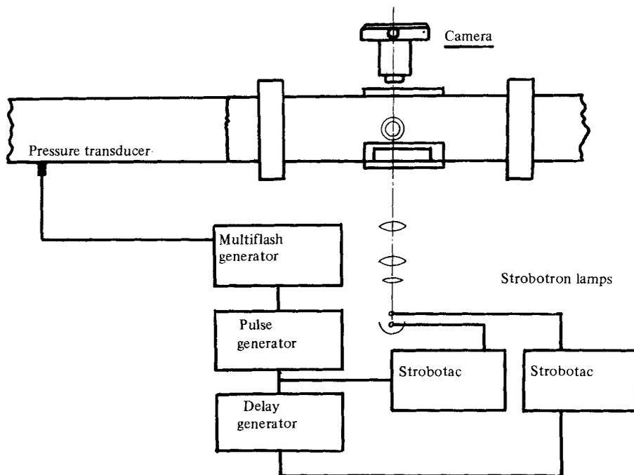
FIGURE 3. Electronic system for flash control.
