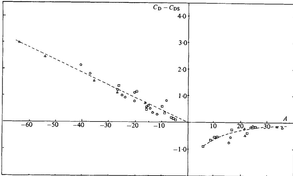
FIGURE 13. Difference between measured drag and steady drag as a function of  $A$  for the data shown in figure 12.
