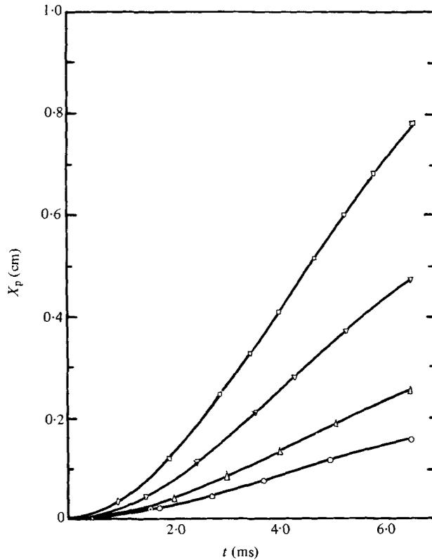
FIGURE 7. Horizontal displacement of  $135 \mu\text{m}$  droplets in several tests.  $\square$ ,  $U_{\text{max}} = 305.6 \text{ cm/s}$ ;  $\triangle$ ,  $403.7 \text{ cm/s}$ ;  $\nabla$ ,  $704.3 \text{ cm/s}$ ;  $\square$ ,  $985.6 \text{ cm/s}$ .
