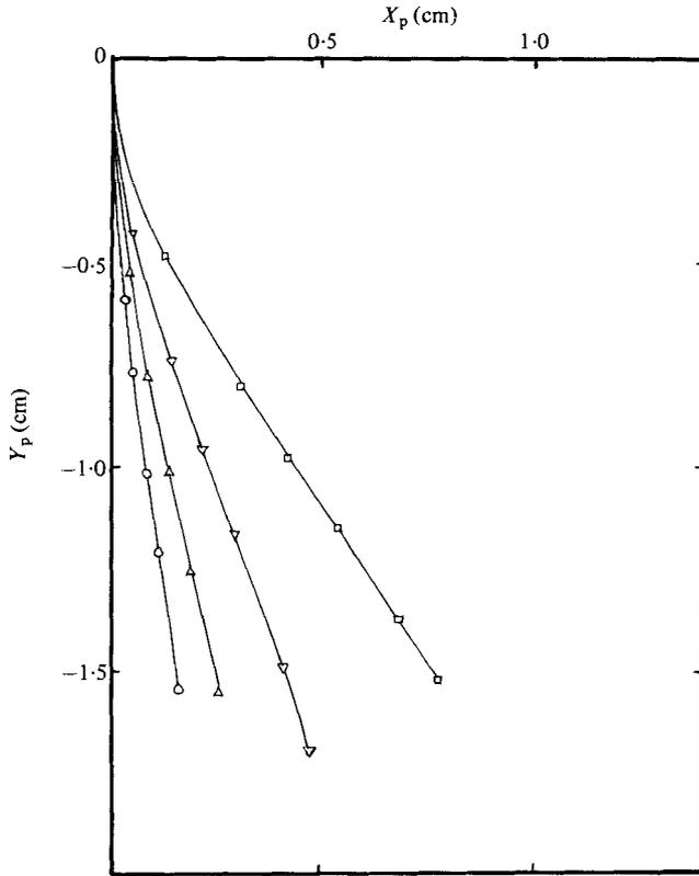
FIGURE 5. Trajectories of  $135 \mu\text{m}$  droplets.  $\circ$ ,  $U_{\text{max}} = 305.6 \text{ cm/s}$ ;
