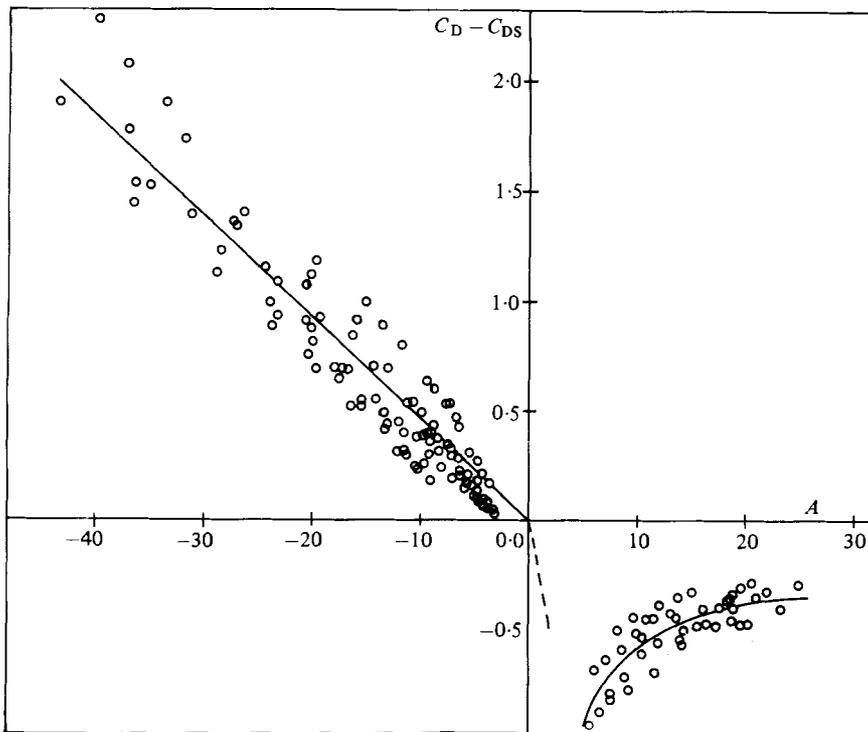
FIGURE 14. Difference between measured drag and steady drag as a function of the relative-acceleration parameter for all of the data having an estimated error in the Reynolds number smaller than 15%.
