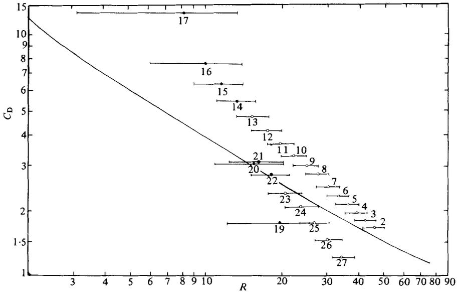
FIGURE 10. Drag-coefficient data for test no. 2514. The data for data-point no. 18, are  $C_D = 127.4$ ,  $R = 2.31$  (see table 2). Data denoted by filled symbols have estimated Reynolds-number errors larger than 15%.
