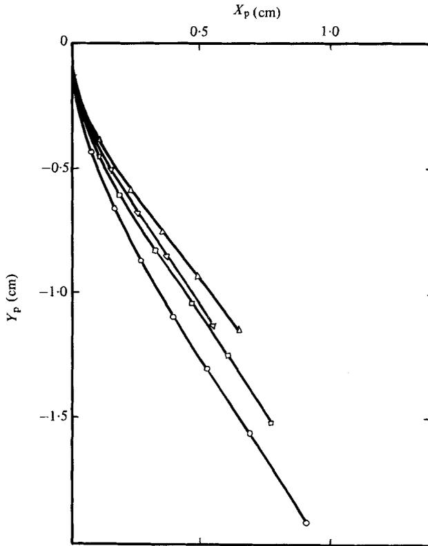
FIGURE 6. Trajectories of different-sized droplets in N-waves having nearly equal maximum velocities,  $U_{max} \approx 990$  cm/s.  $\circ$ ,  $D = 120 \mu\text{m}$ ;  $\square$ ,  $135 \mu\text{m}$ ;  $\triangle$ ,  $167 \mu\text{m}$ ;  $\nabla$ ,  $183 \mu\text{m}$ .
