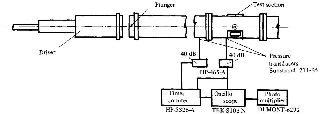
FIGURE 1. Conical-driver shock-tube facility.
